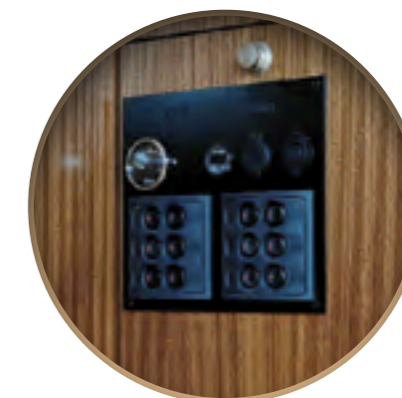
BEP board on engraved PLEXI (With unit name + holes for indicators)
